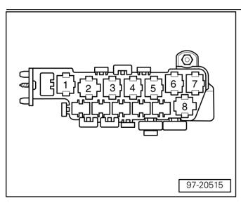
Relay arrangements on eightfold (eight posion) auxiliary relay panel behind relay panel
