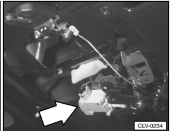
**V151 Motor for remote unlock rear lid**
