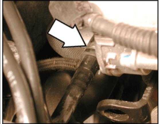
**G2 Engine Coolant Temperature (ECT) Gauge Sensor (2.0 ltr. tdi engine)**
