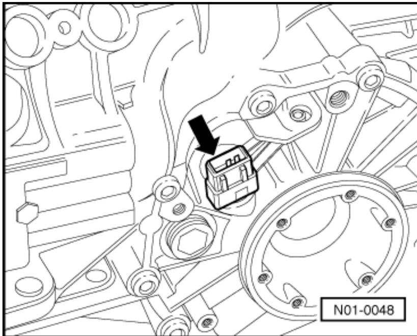
**G22 - Speedometer Vehicle Speed Sensor (VSS)**
