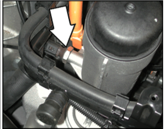
F1 Oil Pressure Switch (2.0 ltr. tdi engine)
