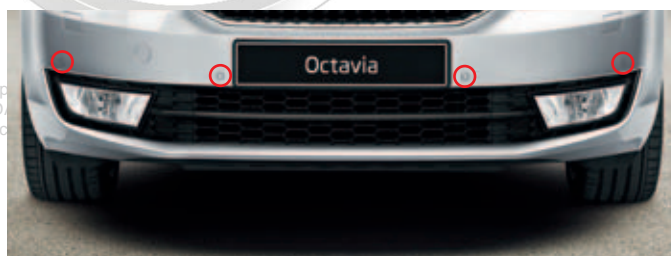
PDC sensor locations in the front bumper
