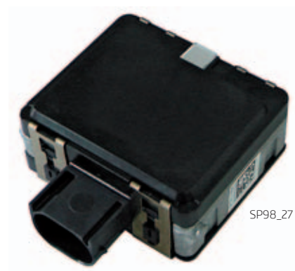
Front radar unit
