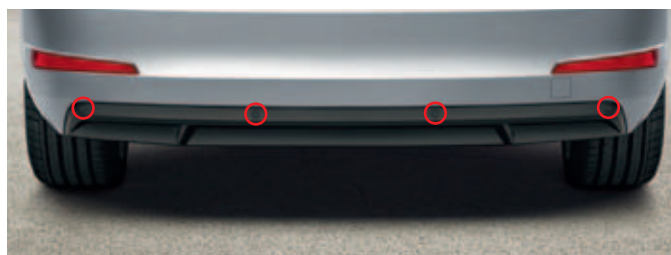
The PDC sensor locations in the diffuser, which is part of the rear bumper
